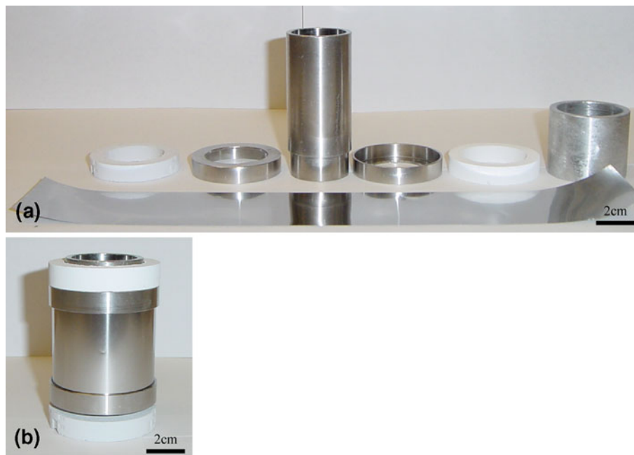
Fig. 3 (a) Customized crucible components shown with representative sample (far right) prior to assembly. Note the 0.25 mm thick stainless steel foil which forms the outside diameter of the sample. This exemplary crucible design is used for a variety of melting, solidification, and heat treatment experiments. (b) Fully assembled UMSA test sample used for advanced heat treatment experiments
