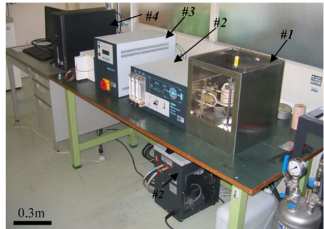
Fig. 4 Universal Metallurgical Simulator and Analyzer UMSA (Ref 28) used for thermal analysis and advanced heat treatment experiments (courtesy of Yamaha Motor Co. Ltd. in Japan). The main system's components are as follows: #1: Testing chamber, #2: Control unit, #3: Induction heating power supplier, and #4: Computer and data acquisition unit
